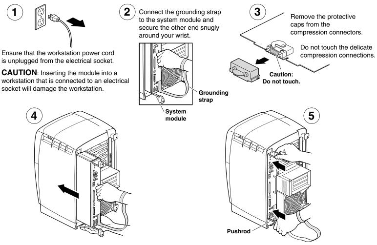
While you support the module with one hand and grasp the handle with the other, slide the system module into the workstation. Push the module completely into the chassis, flush with the I/O panel.
