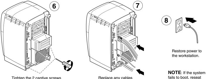
Tighten the 2 captive screws that secure the pushrods.
