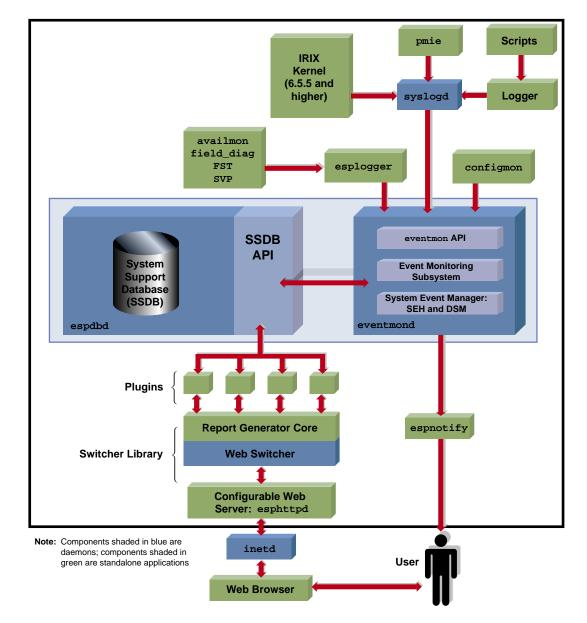
Figure 1-1 Embedded Support Partner Architecture (Block Diagram: Single System)
